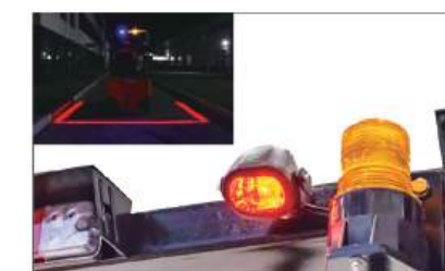
Red Safety Area Lights
